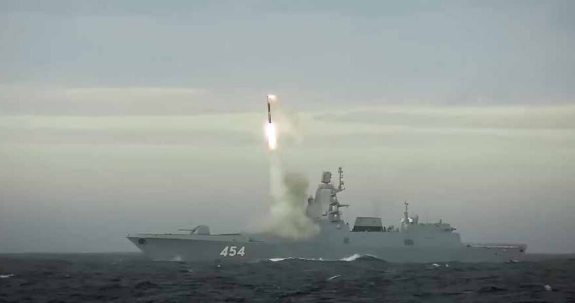
Potential threat and technological benchmark: A Russian frigate launching a 3M22 Zirkon type hypersonic anti-ship missile; May 2022 (source: Youtube/Forces News, 04 Jan 2023; retrieved on 08 Feb 2023)
